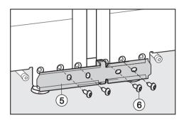
Screw lower bracket (5) securely into position using screws (6).
